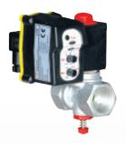
Should the valve still get clogged you can service it without removing from the installation. Press the knob at the bottom of the valve to mechanically clear all the sludge. Electronically flush a few times and now it is fully serviced and ready for use.
