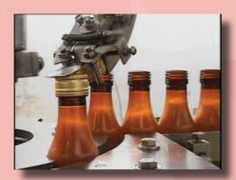
Compressed air may be used to produce linear motion using pneumatic cylinders. Such cylinders are extensively used in applications where there is a high degree of automation, such as bottling plants. Pneumatic cylinders may be used in machines that fit caps on bottle tops and affixing labels on bottles.
