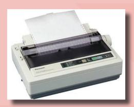
The use of electricity to produce linear motion is restricted to applications in which the forces are small and the travels are short. The solenoids used in electric latches and calling bells provide examples of linear motion produced using electricity. The print heads of dot matrix printers are another example.
