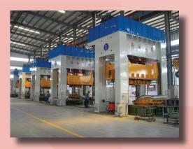
When high pressures or long travels are required, such as in the large presses used to make car bodies, hydraulic systems are preferred.
