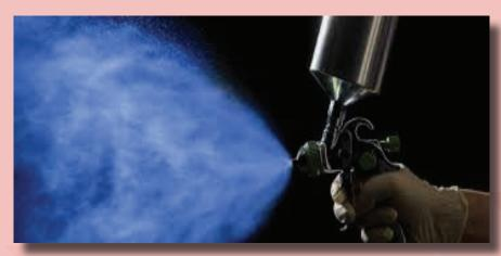
Compressed air has, of course, many other kinds of applications, such as pneumatic conveying of powders, spraying powder in powder coating processes, spraying liquids in painting and inflating tyres. Electrical or hydraulic alternatives are not available for all these applications.
