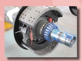
Another example of the production of linear motion using compressed air is seen in air brakes, where brake shoes are pressed against brake drums pneumatically.
